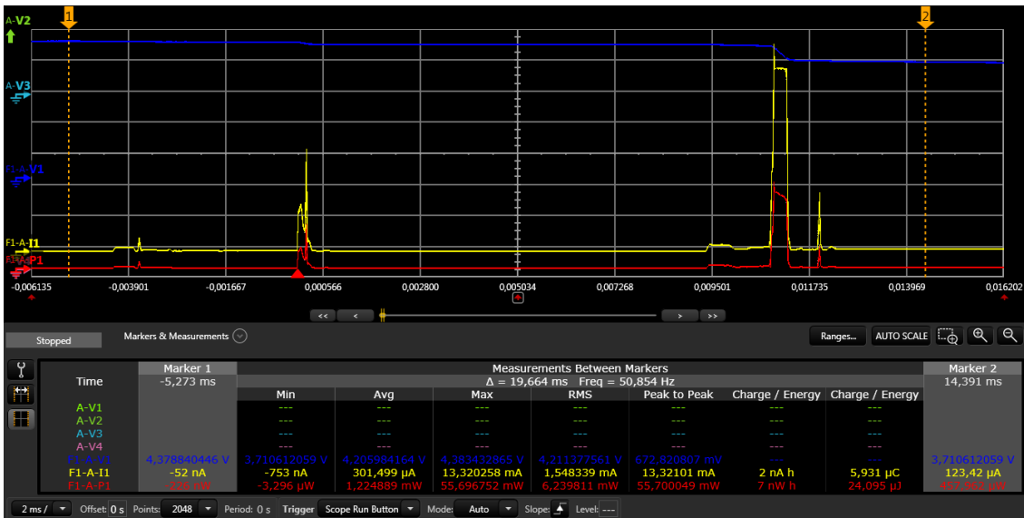
Fig. 8. 10μF storage. Frame is enough for Ble. 1 ADV sent /1v/div, 2mA/div, 20mw/div). Whole system starts around 4.4V and works down to 3.7 volts. 24μJ measured.
