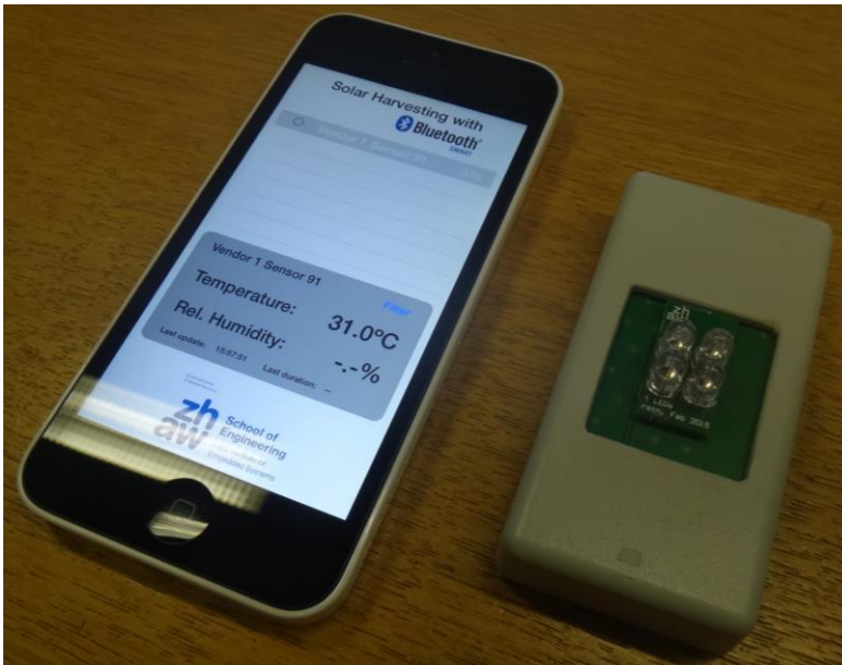
Fig.12. Sensor powered by 4 LEDs sending data to a smartphone
