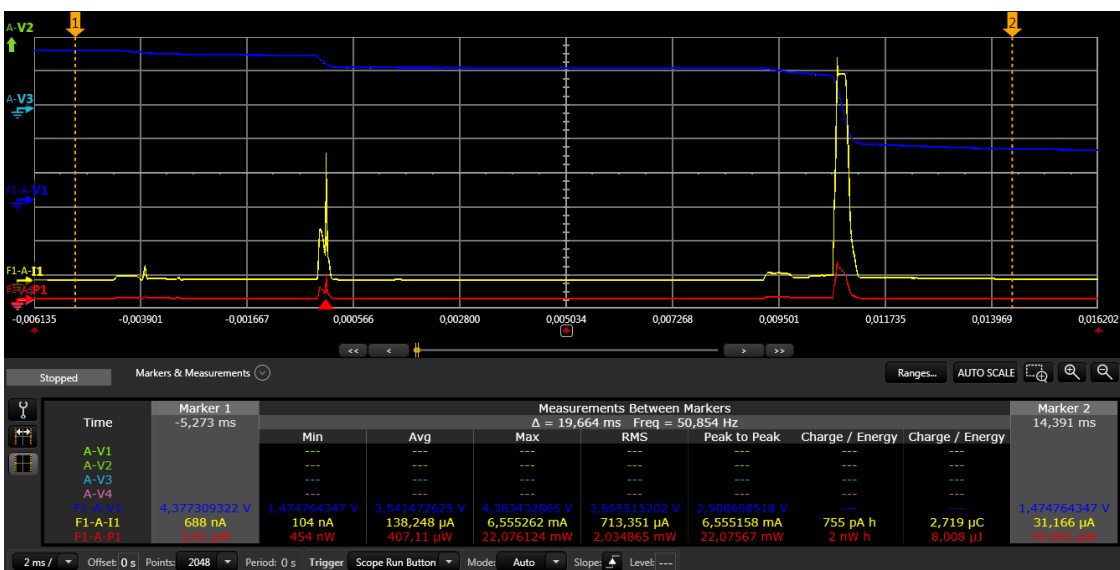
Fig. 7. 1-2 \mu F storage in system. Not enough energy for a Ble frame. The frame is wrongly transmitted (last parts truncated because there is not enough energy). But the available energy will be enough for the short frame in the proprietary system.
